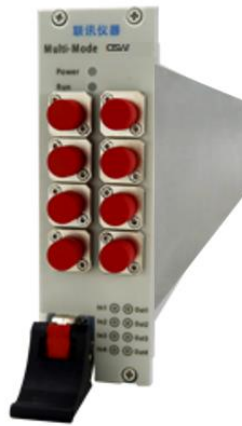
Fig. 6 Multi-mode 1x4 optical switch
